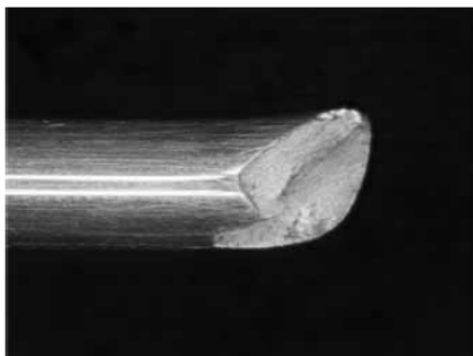
Broken Aluminum Wire
